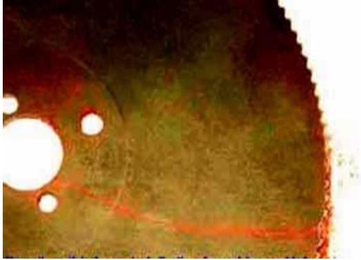
Indication of a crack in a saw blade
