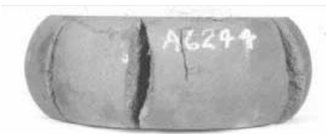
Multiple forging bursts in a steel blank
