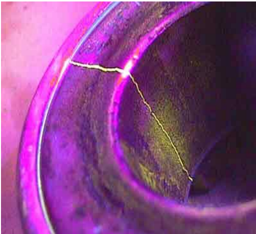
Magnetic particle wet fluorescent indication of a crack in a bearing
