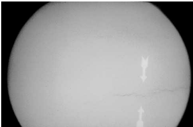
Radiograph of hot tear in a casting
