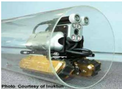
Remote visual inspection using a robotic crawler.
