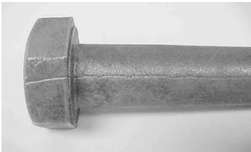
Crack in bolt
