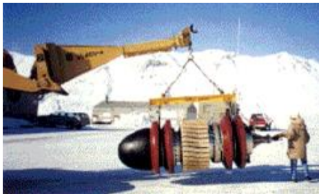
Magnetic flux leakage inspection. This device, known as a pig, is placed in the pipeline and collects data on the condition of the pipe as it is pushed along by whatever is being transported.
