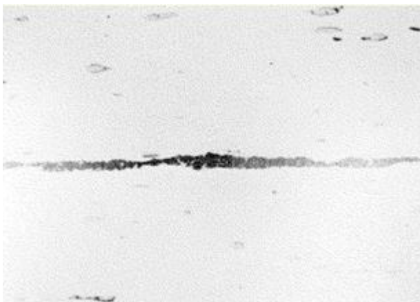
Silicate stringer in cold drawn bar of steel (235X)
