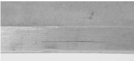
Lamination in plate edge
