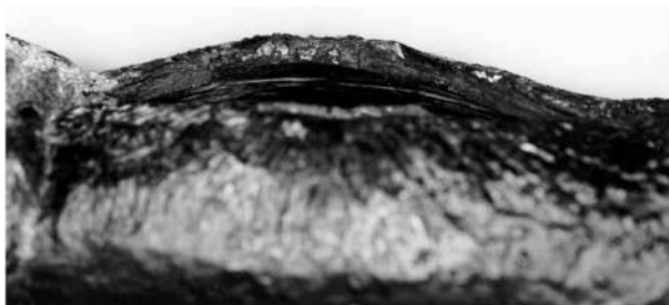
Thick lip fracture from creep in a power plant superheated tube
